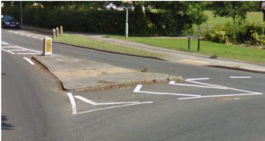
Image 8: Example of flared road marking at roundabout, reducing roundbaout circulatory.
